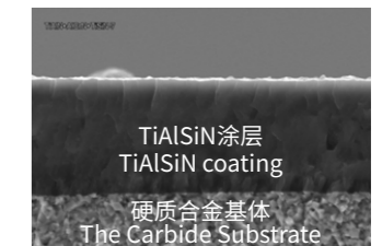
涂层断面形貌 SEM Photograph of Coating
